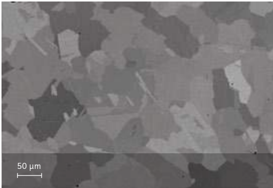
Microstructure from Heat Treatment Option 1. Oxalic acid etch, section perpendicular to building direction.
