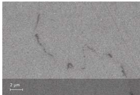
Microstructure from Heat treatment Option 2. Oxalic acid etch, section perpendicular to building direction.
