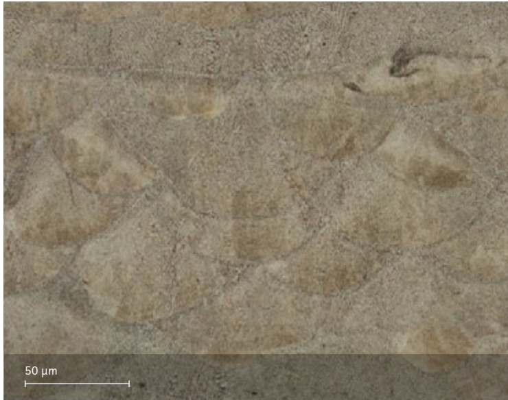
As manufactured microstructure. Etchant: Kalling's II
