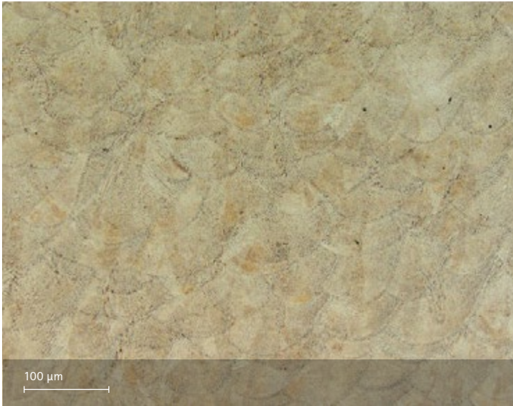
As manufactured microstructure. Etchant: Kalling's II
